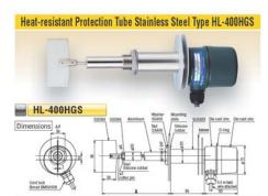
Model with long length for dimension L. High-temperature model able to withstand temperatures of up to 100°C. Parts that come into contact with powder are made of stainless steel. Available lengths for dimension L are 150, 200, 250. or 300 mm.
